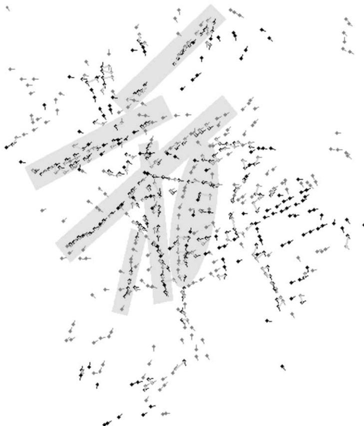
Fig. 2. Feature point matchings (both point positions and orientations are matched) corresponding to the palmprint pair in Fig. 1(i). The 153 point correspondences found are shown using light gray segments. The six main palm lines which have been matched are shown inside the solid gray areas. Due to a different position of the thumb in the two palm scans, the diagonal palm lines inside the ellipsoidal area differ by a non-linear transformation.
